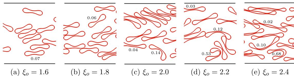
**Fig. 4** Visualizations showing the onset of apparent buckling behavior for  $H_c = 0.25$ ,  $W = 14r_o$ ,  $u^* = 1.0$  for  $\xi_o$  as labeled. The inset numbers indicate the buckling metric defined in “Buckling”
