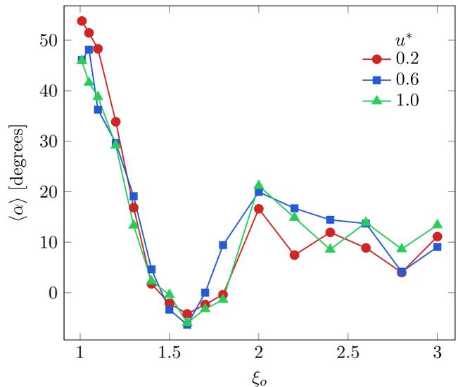
**Fig. 10** Mean orientation angle for varied  $\xi_0$  and flow strengths  $u^*$ .  $H_c = 0.25$  and  $W/r_0 = 20$  for all cases
