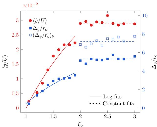
**Fig. 16** The average transverse velocity of the capsules ( $\dot{y}/U$ ) and transverse displacement  $\Delta_y/r_o$  from Eq. 19. We also show  $\Delta_y$  for exclusively capsules that have buckled at least once during the course of the simulation,  $(\Delta_y/r_o)_b$
