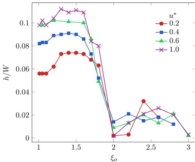
**Fig. 8** Dependence of the capsule-free layer thickness on  $\xi_0$  and capillary number  $u^*$ , shown for cases with  $W/r_0 = 20$  and  $H_c = 0.25$
