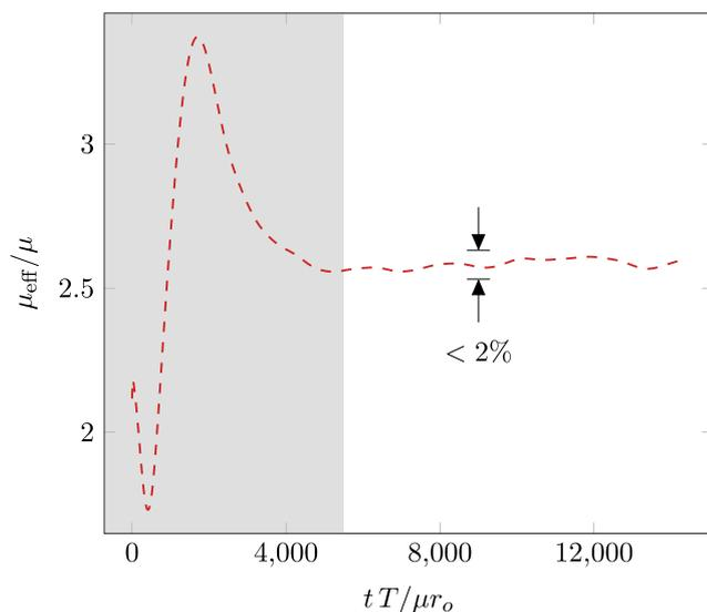
**Fig. 5** Instantaneous  $\mu_{\text{eff}}$  from Eq. 12 for  $H_c = 0.25$ ,  $W = 20r_o$  and  $\xi_o = 2.4$ . The nominally transient period is shaded, after which effective viscosity deviates by  $< 2\%$
