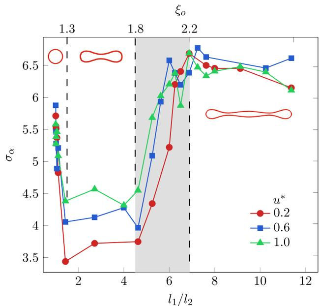
**Fig. 11** Variance of orientation angle  $\sigma_\alpha$  as a function of configuration aspect ratio and capillary number for  $W/r_0 = 20$  and  $H_c = 0.25$ . The vertical dashed lines represent approximate geometry and behavioral regimes as indicated
